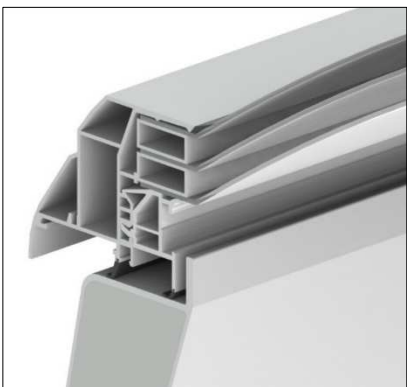
Triple skin construction U_t approx. 1,8 W/m 2 K
